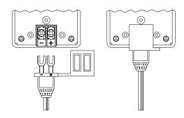
If using loose wires, insert stripped ends under washers. A cable having a shield may be grounded to the bottom hole using a number  $6-32 \times \frac{1}{4}$  machine screw.
